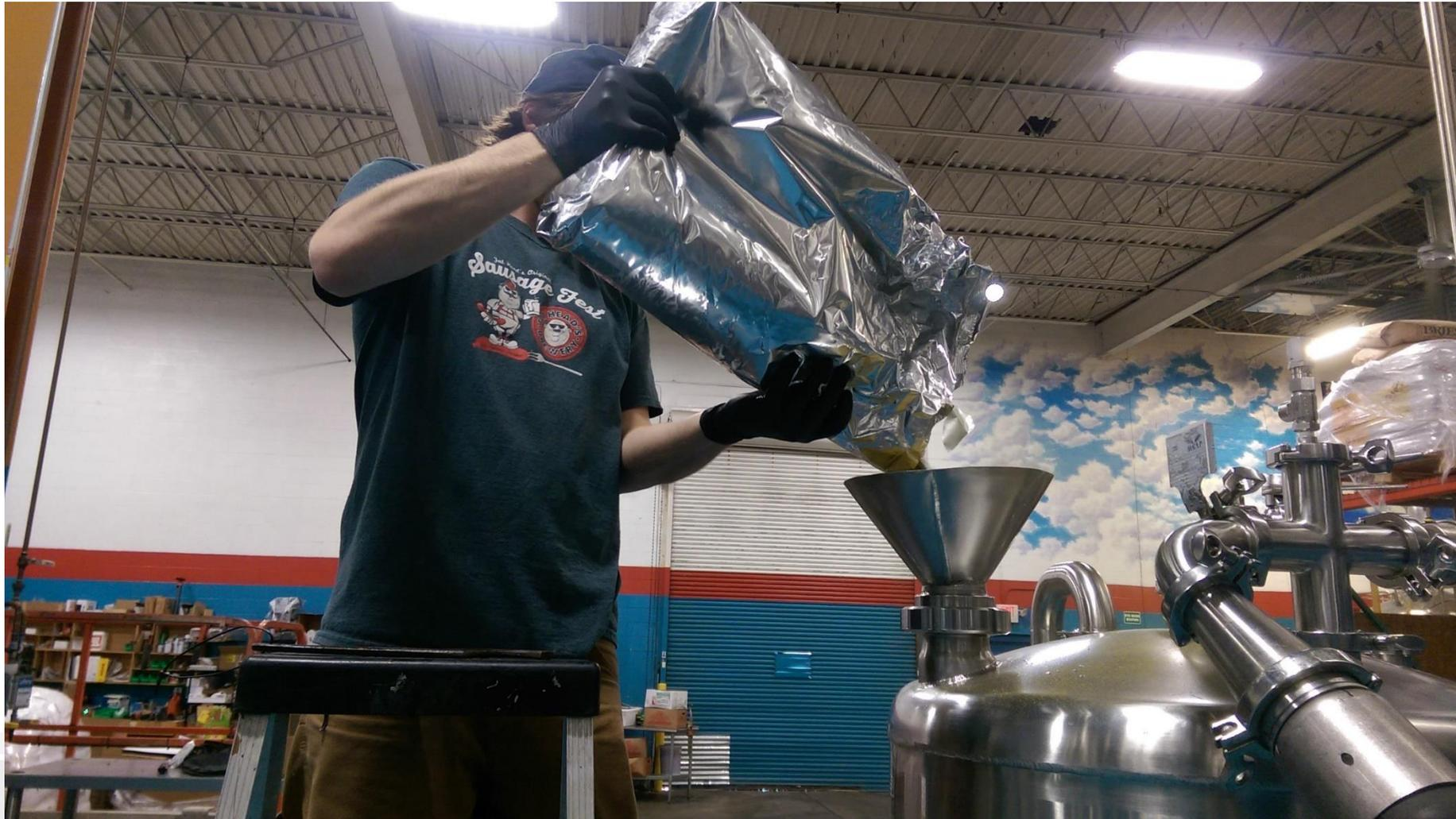
Once hops are loaded, funnel is removed and port closed. Switch CO<sub>2</sub> to back port.
