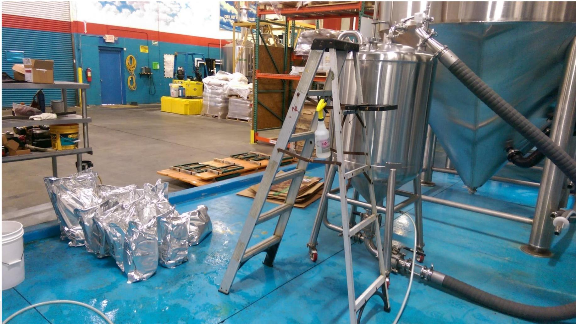
Close up of CO<sub>2</sub> connection. Creates CO<sub>2</sub> Blanket for loading hops.
